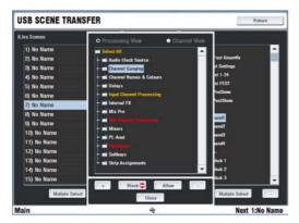
To select and transfer Scenes from the USB key go to the UTILITY / Configuration / USB Scene Transfer page. Plug in the USB key. All Shows found on the key are listed in the right hand window. Highlight a Show and touch the + button to open up the list of Scenes in that Show.
